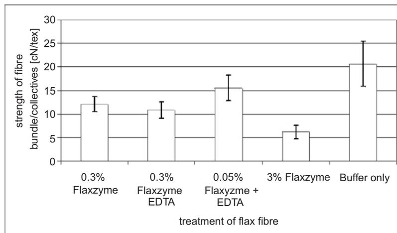
Comparing the strength of enzymatically separated flax fibre bundles with Flaxzyme (Fig. 8, Akin et al., 1999) and enzymatically separated hemp and nettle fibre with BioPrep3000L<sup>®</sup>, we found much higher strength ratings in our trials for both plants. The micronaire for flax fibre of between 4.3 and 8.0 did not explain the loss in strength (Akin et al., 1999). Some reasons for these differences could be variations in raw material, enzyme formulation, and conditions.
