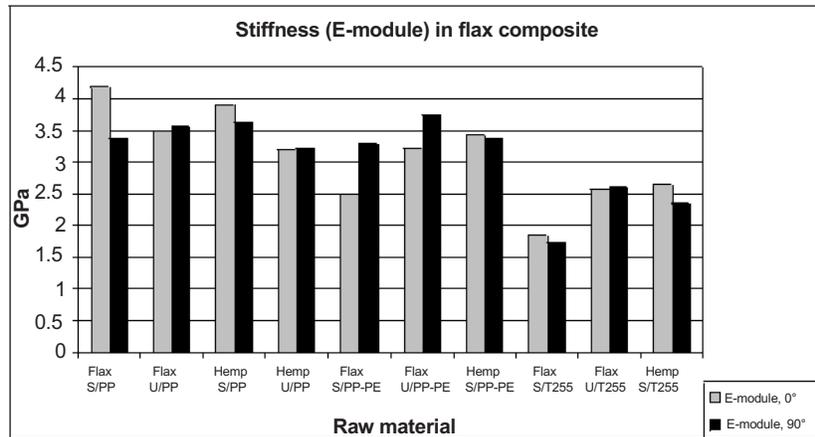
In comparison to the stiffness and strength of the fibres themselves, flax fibres obtain strength in the elementary fibre at 290 MPa in strength and 44 GPa in stiffness (Lilholt and Toftegård, 1999).
