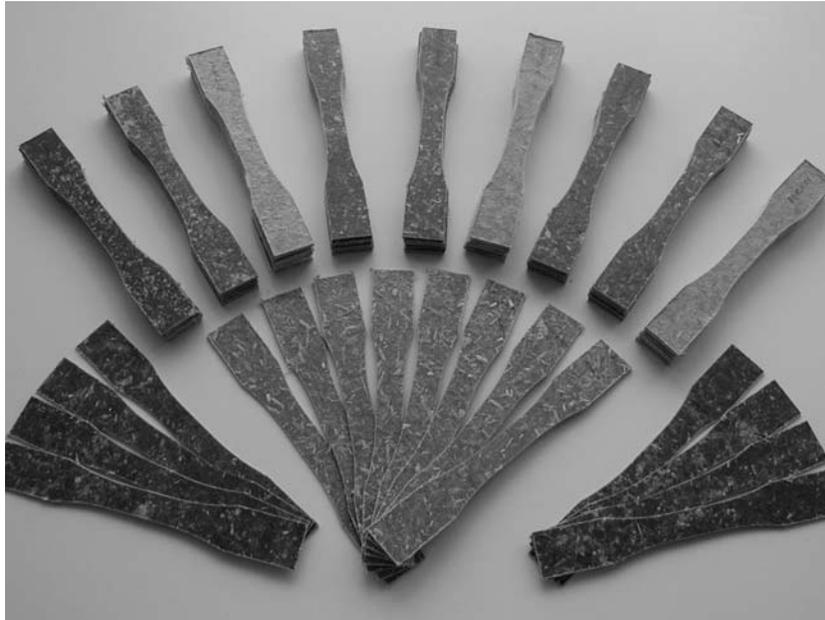
found typically 25%, in jute composite modified with MAPP (Maleic anhydride grafted polypropylene). The improvement is due to a better chemical bonding between the natural fibres and the matrix.
