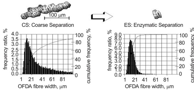
FIGURE 4. OFDA results on chemically and enzymatically separated hemp bundles
