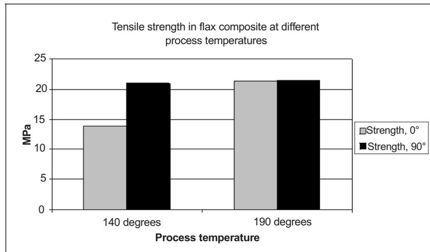
The chosen 50% weight content of plant fibre (from 27%-48% vol.) is relatively high in order to achieve a good adhesion and wetting between fibre and matrix. A higher content diminishes the possibilities to achieve a good fibre wetting due to an insufficient amount of polymer.
